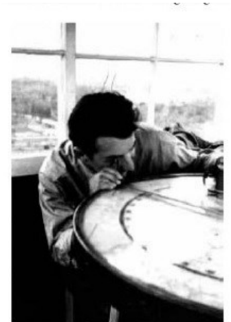
Pete Bond sighting smoke with alidade in Long Hill fire tower in the early 1940s. Photo courtesy Jenny Bond in "A History of Green Ridge State Forest," 2010.
