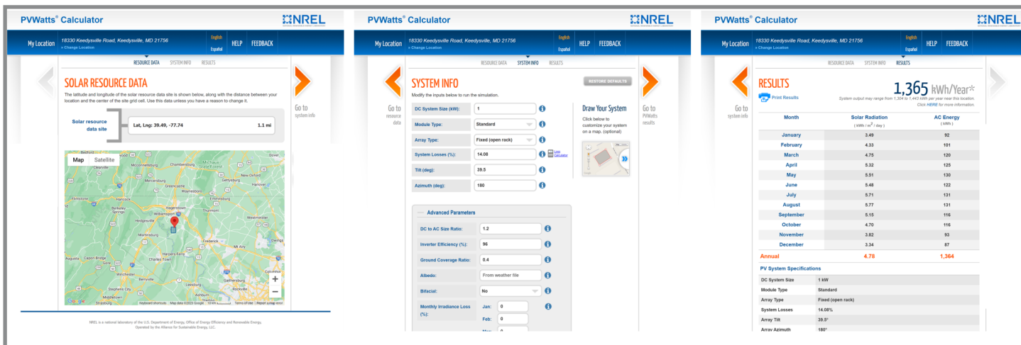
Figure 11. System sizing for a fixed-open rack system located in western Maryland using PVWatts (NREL, 2023). The output under optimal conditions indicates a single kW of solar PV panels will produce 1,365 kWh per year. System capacity (kW) is calculated by dividing annual energy demand (kWh) by this estimation of annual energy production (kWh per kW).
