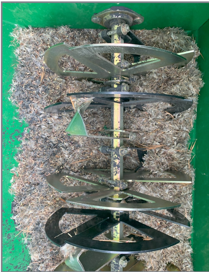
Figure 5: Agitator wheels in the seed box of a native seed drill that slowly rotate to facilitate seed dropping into planting tubes. Photo by Luke Macaulay.
