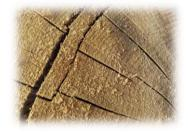
Figure 5. "Checking" of firewood
