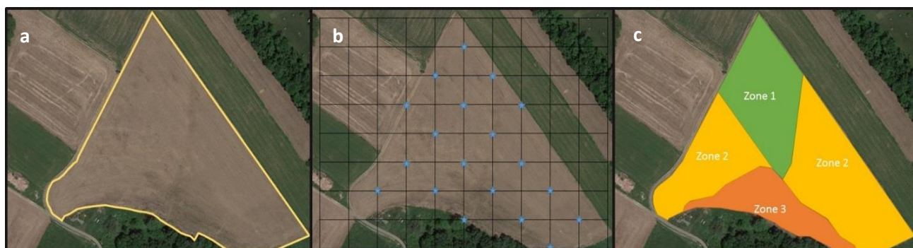
Figure 1. Soil samples may be collected for the (a) whole field, (b) on a consistently spaced grid or (c) by management zones
