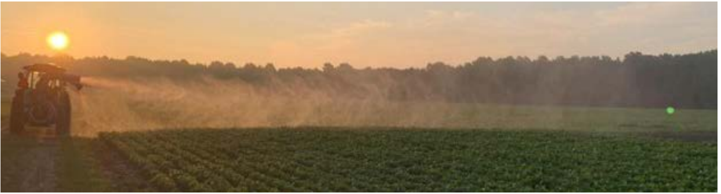
Figure 12: Air-blast sprayer can apply repellents over one hundred feet into a field without having to enter the field. Photo by Luke Macaulay.
