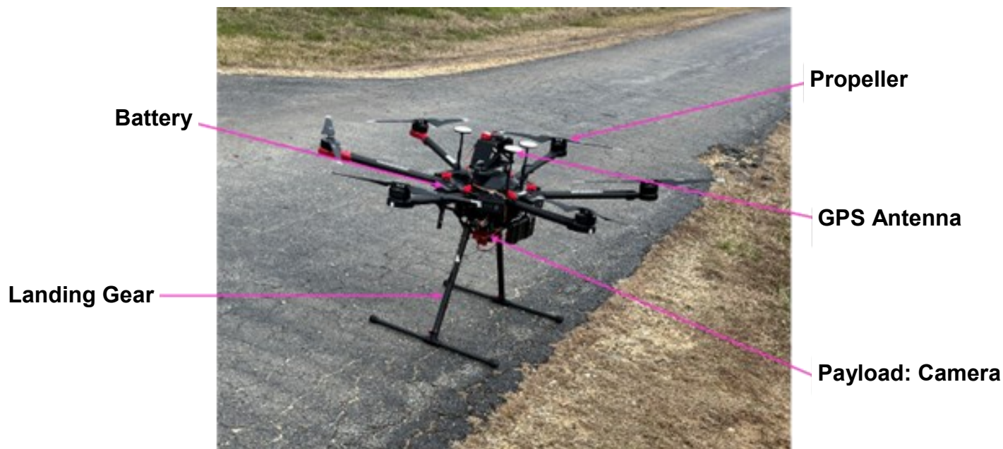
Figure 2. Different components of a typical drone. (Photo by H. Kumar, University of Maryland)
