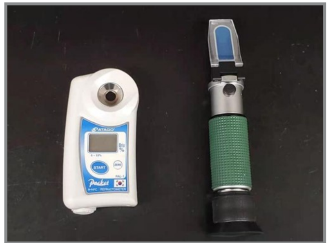
Figure 6. A hand-held manual refractometer (right) and digital refractometer (left) for measuring soluble solids contents of extracted peach juice sample. Source: Yixin Cai, University of Maryland
