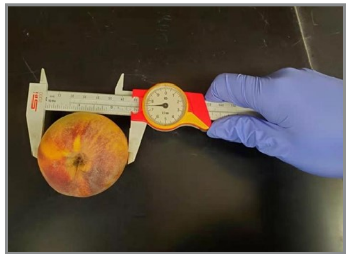
Figure 4. Using a hand-held caliper to measure the diameter of peach. Source: Yixin Cai, University of Maryland
