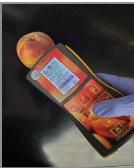
Figure 3. Using a DA meter to quantify the Index of Absorbance Difference ( I_{AD} ) in peaches which relates to the actual content of chlorophyll-a in the fruit skin. Source: Yixin Cai, University of Maryland
