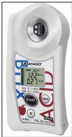
Figure 7. ATAGO pocket Brix-Acid meter determines total soluble solids and titratable acidity for apples. Photo: ATAGO ( https://www.atago.net/product/?l=en&f=products-bx-acid-top.php#DCL37705 ).
