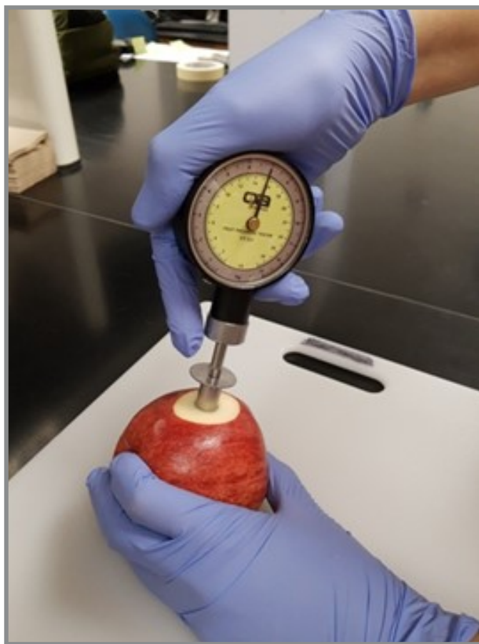
Figure 2. An Effegi firmness tester/penetrometer with a 7/16-inch diameter plunger used to measure firmness in one side of an apple.
