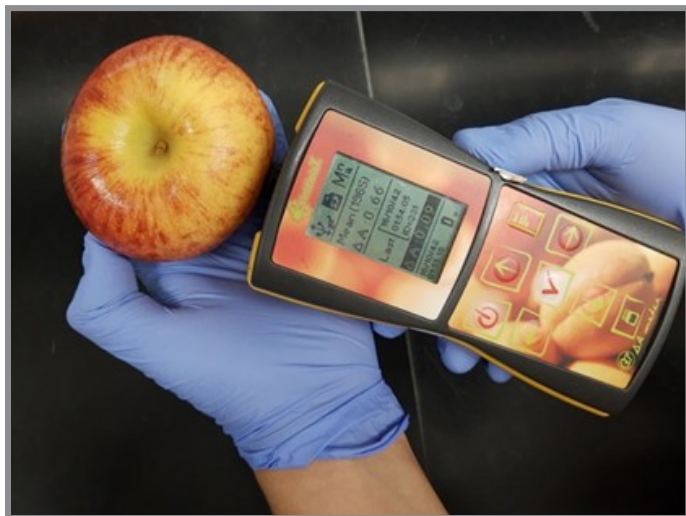
Figure 1. Using a DA meter to quantify the Index of Absorbance Difference ( I_{AD} ) which relates to the greenness and thus content of chlorophyll-a in the fruit skin.
