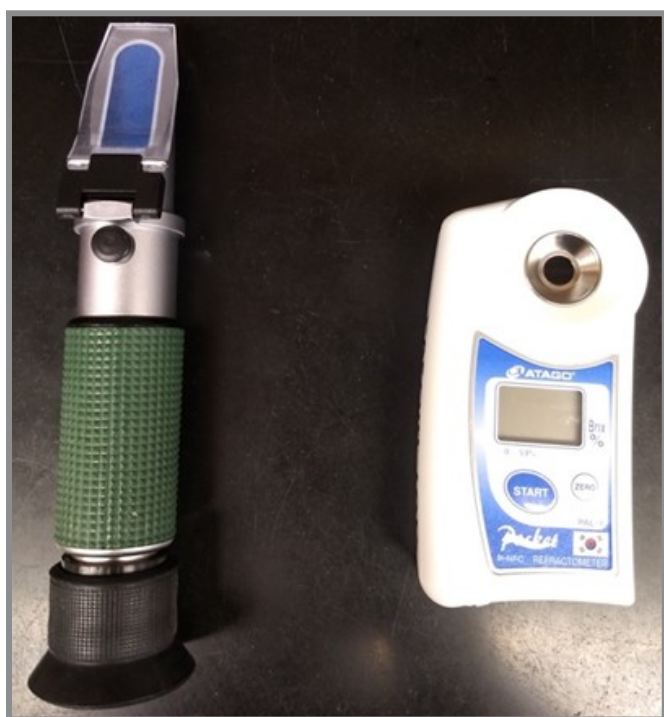
Figure 6. A hand-held manual refractometer (left) and digital refractometer (right) measure soluble solids contents of an extracted fruit apple juice sample.
