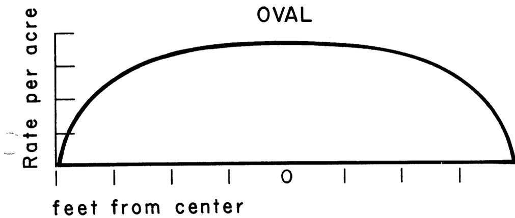
Figure 6. The normal spreader distribution.
