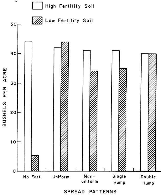
Figure 2. The effect of fertilizer spread patterns on the yield of wheat (VPI & SU, 1970).
