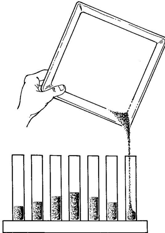
Figure 4. The spread pattern is easily seen when the trays are emptied into tubes.
