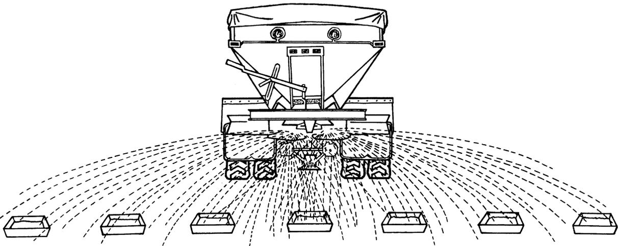
Figure 3. The tray system for evaluating spreader distribution pattern.
