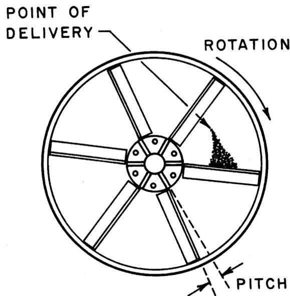
Figure 9. Adjustment of point of fertilizer delivery, blade pitch or spinner speed may be necessary for uniform distribution.
