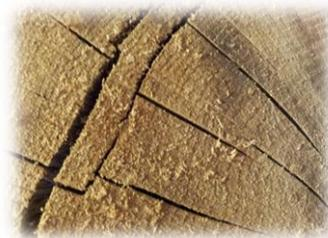
Figure 5. “Checking” of firewood
