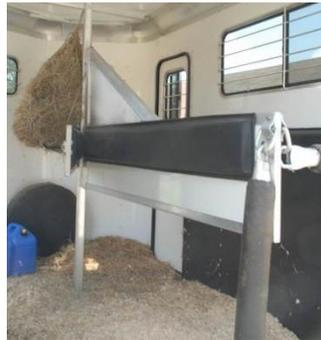
*Partial divider and butt bars in a straight load trailer.*
