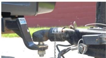
*A bumper pull trailer attached to the hitch.*
