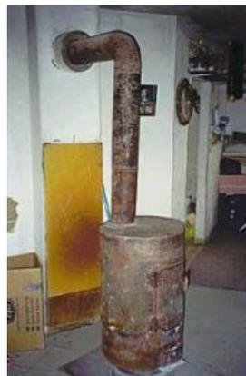
*An example of a stove showing signs of metal fatigue, probably from being repeatedly overfired.*
