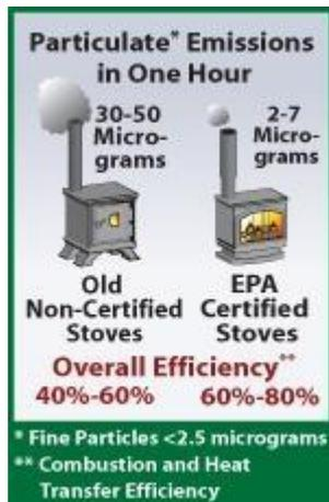
*A stove that is 30% more efficient saves 30% in fuel costs and/or time cutting, splitting, stacking and moving it.*
