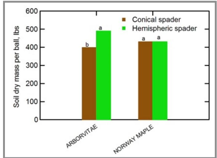
Figure 3. Amount of soil removed in 32 inch diameter tree root balls. For Arborvitae, tree harvester type affected the amount of soil removed. The point of the conical root ball (Caretree spade) is knocked off, removing a varying amount of soil from the root ball. The hemispherical root ball (produced by Pazzaglia spade) is bowl shaped and not normally altered before wrapping. N=12.
