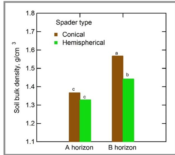
Figure 6. Soil bulk density in A and B horizons (topsoil and subsoil) of root balls for two spade types. Means of two tree species. n=12.
