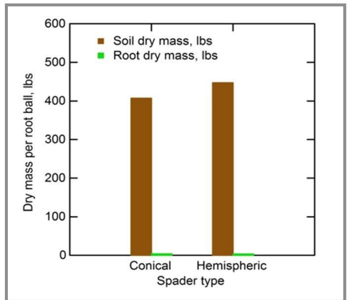
Figure 4. Dry weight of soil and root material in tree root balls made by two types of spade. The dry weight of the roots was negligible compared to that of the soil in each case. N=12
