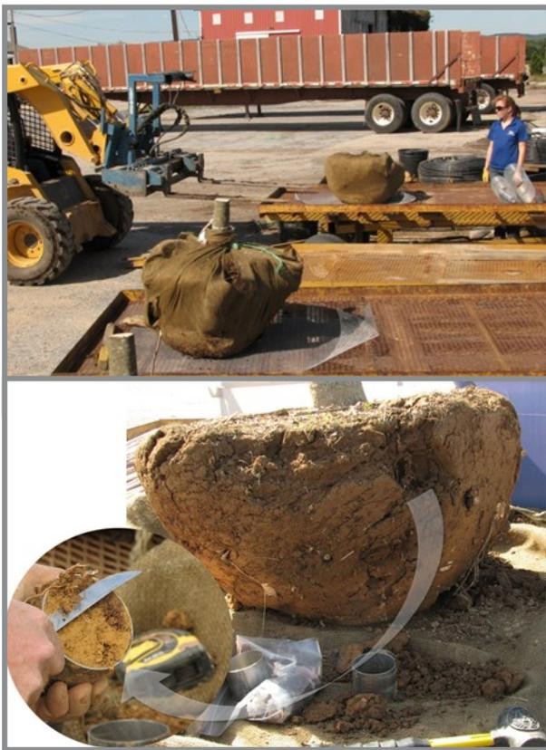
Figure 1. (top) Preparing tree balls for analysis at the nursery. (bottom) Taking bulk density core from tree ball prior to separation of roots and soil. (Photos by R. Weil).
