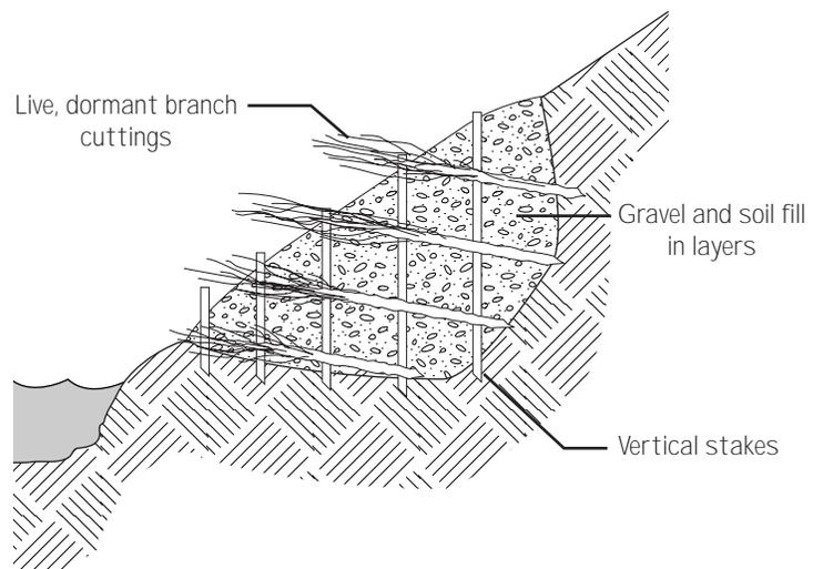
An adaptation of several of the above techniques is brushmattressing (Figure 6). It is fairly involved and labor-intensive to construct, but benefits are both immediate and long term. After any needed grading is done, a live fascine is placed at the toe of the slope. Upslope from the fascine a grid of alternating dormant and dead stakes are driven into the ground. Around these stakes a layer of live, dormant, untrimmed branches are laid to cre-
