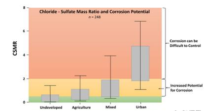
Corrosion potential based on Chloride to Sulfate Mass Ratio (CSMR) for various land uses.
