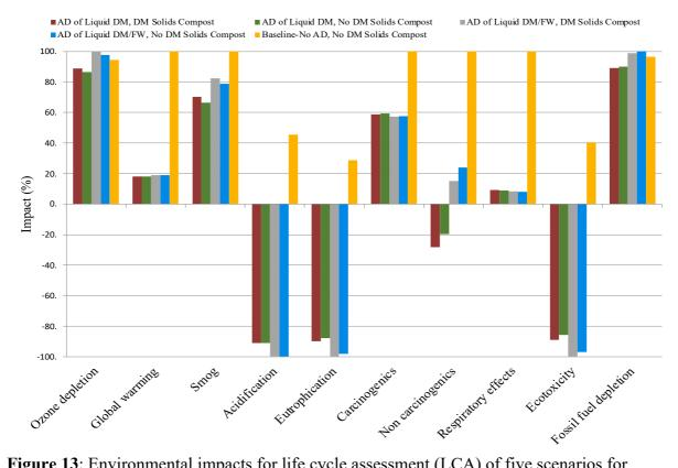
**Figure 13**: Environmental impacts for life cycle assessment (LCA) of five scenarios for farm-scale anaerobic digestion (AD) of dairy manure (DM), food waste (FW) and composting of dairy manure solids with a functional unit of one year.
