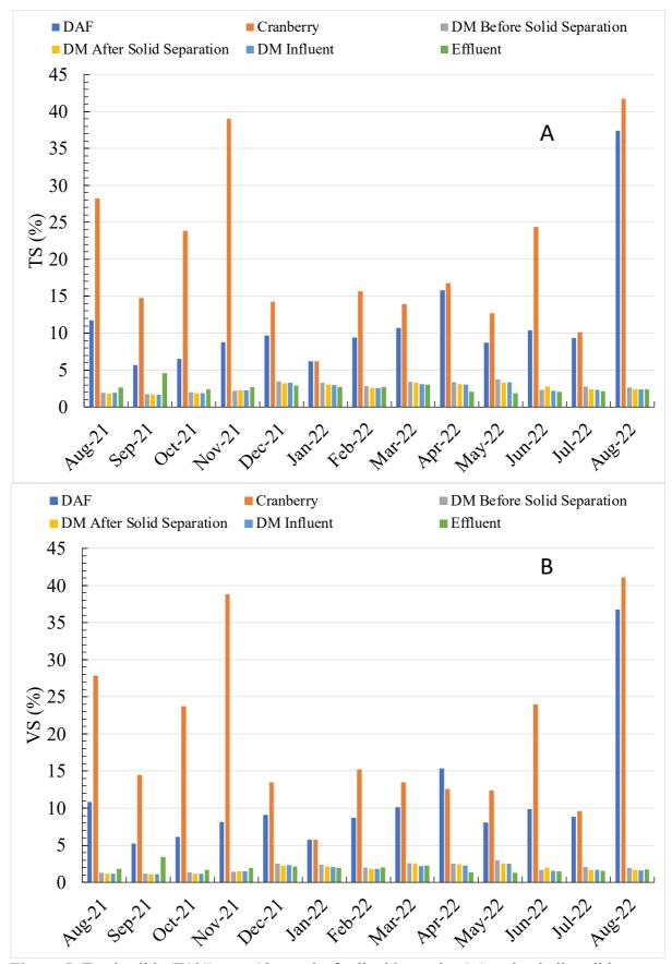
**Figure 5**: Total solids (TS%) over 13 months for liquid samples (A) and volatile solids (VS%) for liquid samples (B) over the sampling period.
