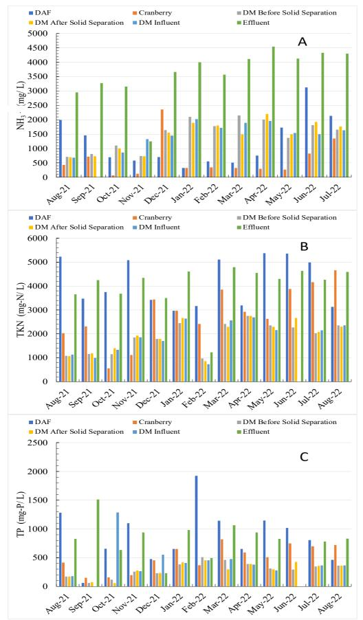
**Figure 7:** Average ammonia (NH<sub>3</sub>) (A), total nitrogen (TKN) (B), and total phosphorous (TP) (C) concentrations for liquid samples over the sampling period.
