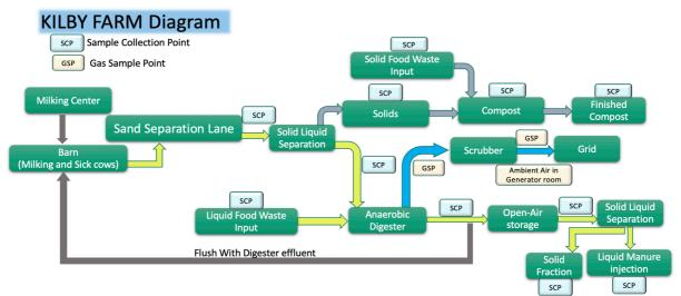
Figure 1: The solid, liquid, and gas sampling points for the AD and composting facilities.
