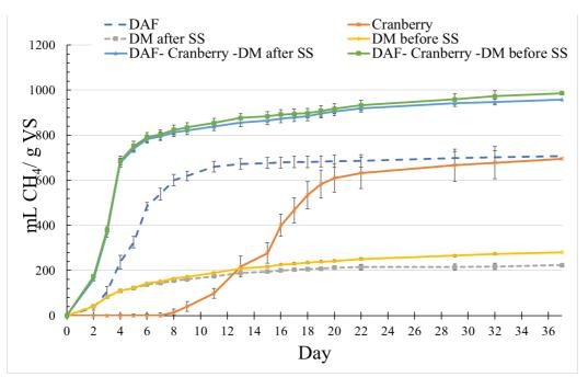
**Figure 11:** Cumulative methane (CH<sub>4</sub>) production based on volatile solids (VS) for poultry processing dissolved air flotation (DAF) waste, cranberry waste, dairy manure (DM) before and after solid separation (SS), and mixtures of these substrates.
