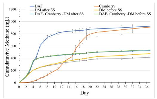
**Figure 12:** Cumulative methane (CH<sub>4</sub>) production for poultry processing dissolved air flotation (DAF) waste, cranberry waste, dairy manure (DM) before and after solid separation (SS), and mixtures of these substrates.
