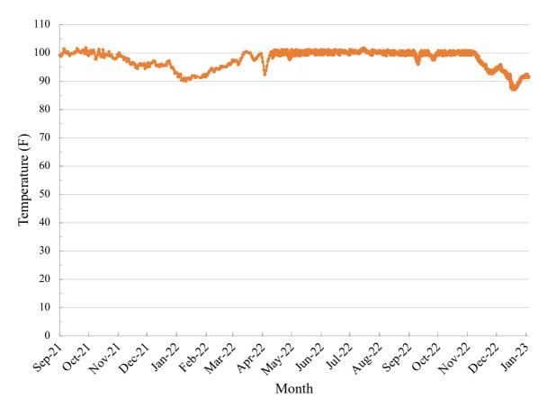
Figure 8: Temperature over the monitoring period for farm-scale AD system (°F).
