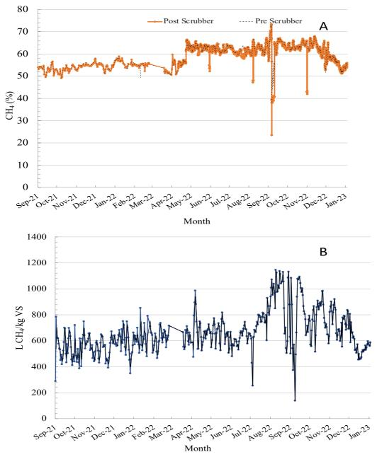
**Figure 2:** The percent methane (CH<sub>4</sub>) in the produced biogas in (A) and CH<sub>4</sub> production normalized by the volatile solids (VS) in the digester influent in (B) from co-digestion of dairy manure and food waste.
