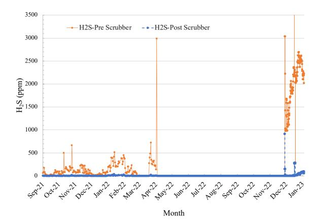
Figure 3: Hydrogen sulfide (H<sub>2</sub>S) concentration in the biogas over the monitoring period.
