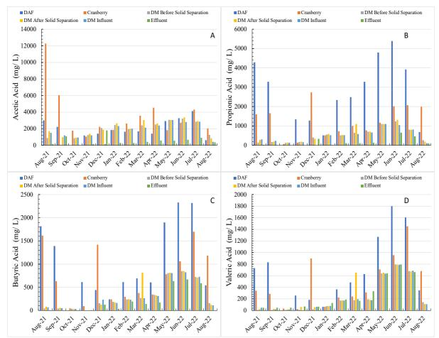
**Figure 10:** VFA concentrations (mg/L) of acetic acid (A), propionic acid (B), butyric acid (C), and valeric acid (D) over the sampling period.
