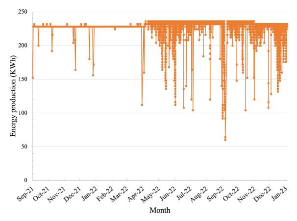
Figure 4: Energy production kWh from the combined heat and power (CHP) generator.
