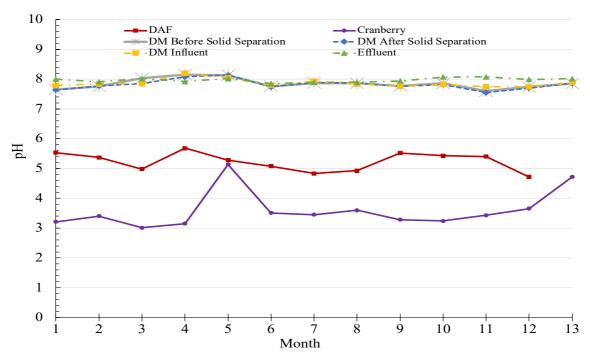
Figure 9: pH for liquid samples over the sampling period.
