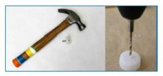
**Step 3** Using either a hammer/nail or a drill, carefully punch a hole through the center of the bottle cap. (in your kits, this is done for you.) This is a key component of the watering system.
