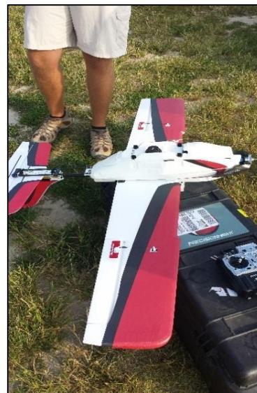
**Figure 3. An example of a fixed wing UAV, which is very similar to an airplane in appearance**
