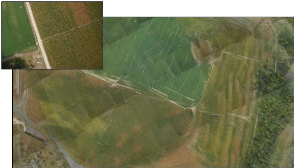
**Figure 6.** One image is easily obtained by a UAV (a). Combining those images into a mosaic of the entire field requires each photo to be marked by a GPS and sophisticated software to stitch them together. Without the software, roads and field boundaries may not line up (b)
