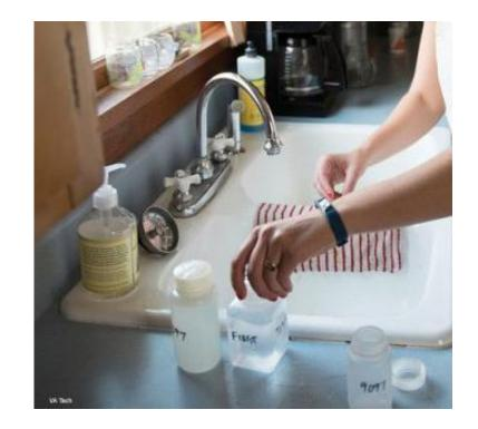
Water quality testing including first draw and 3 minute flush is required to determine influence of corrosion on presence of heavy metals in drinking water.
