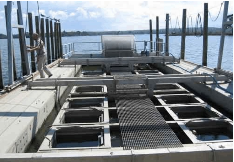
Large paddlewheel FLUPSY in Va
