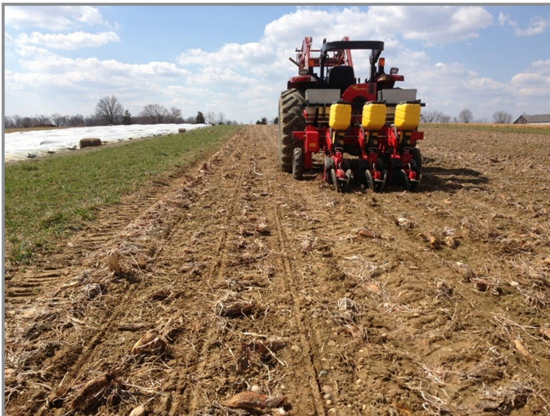
Figure 12. Heavy seeders with coulters and/or double disk openers have no trouble slicing through radish residue. Adjustments may be necessary for adequate furrow closing. Photo: Dave Liker.
