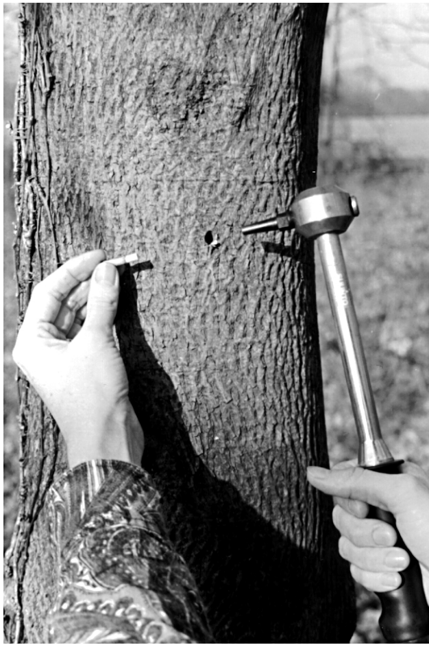
Figure 12. An increment hammer is used to obtain a sample of a tree's outer inch.
