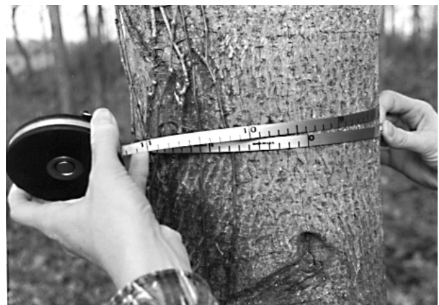
Figure 10. Measuring tree diameter at 4.5 feet from the ground using a diameter tape calibrated to allow direct tree diameter readings in inches.
