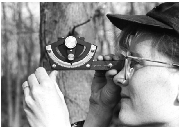
Figure 1. To use an abney level, sight an object through the telescope and move the level bubble to the center position. The number on the scale is the correct reading.
