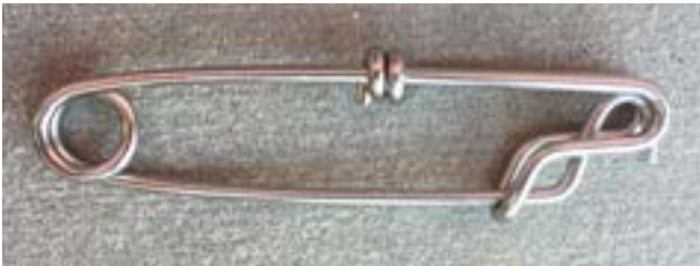
Figure 12. Swordfish/longline clips to secure OysterGro® cages and guy-lines to anchored longline.
