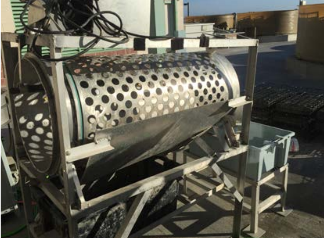
Figure 20. Oyster tumbler used at six-week intervals during processing.
