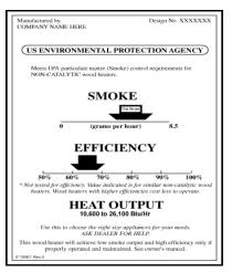
A sampler hang tag that can be found on new EPA certified stoves. Note the measurements for smoke, efficiency and heat output. Unlike the smoke (emissions), the efficiency rating is a very general estimate and cannot be relied on.
