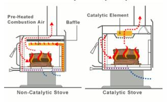
A cross-comparison of a cat and non-cat stove. The cat stove pictured here is an older model that has the catalyst horizontal and directly above the fire. Newer models have them protected from the fire and they are usually vertical.
