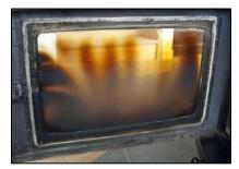
Dirty glass is a tell-tale sign that a stove is not operating the way it should. It usually means the operator is not giving the fire enough air and/or is using unseasoned wood.
