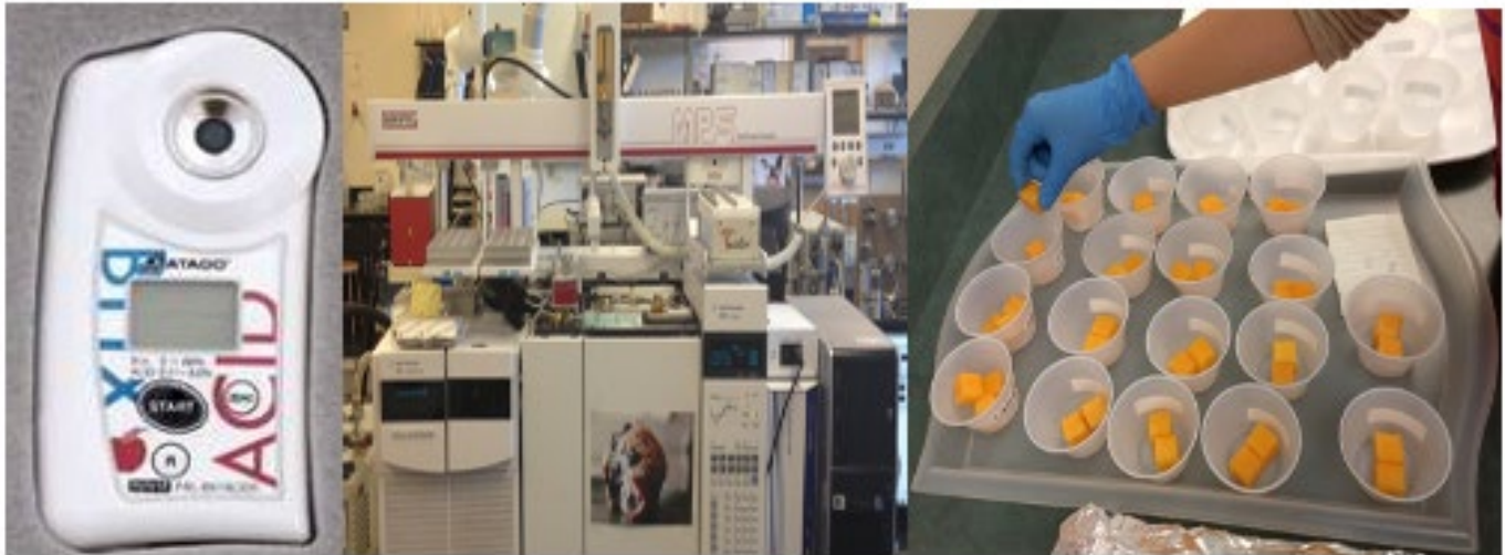
Portable sugar (refractometer) and acidity meter (left); Gas Chromatography – Mass Spectroscopy (GC-MS) equipment (center); samples for sensory evaluation (right). Photo: Dr. Macarena Farcuh
