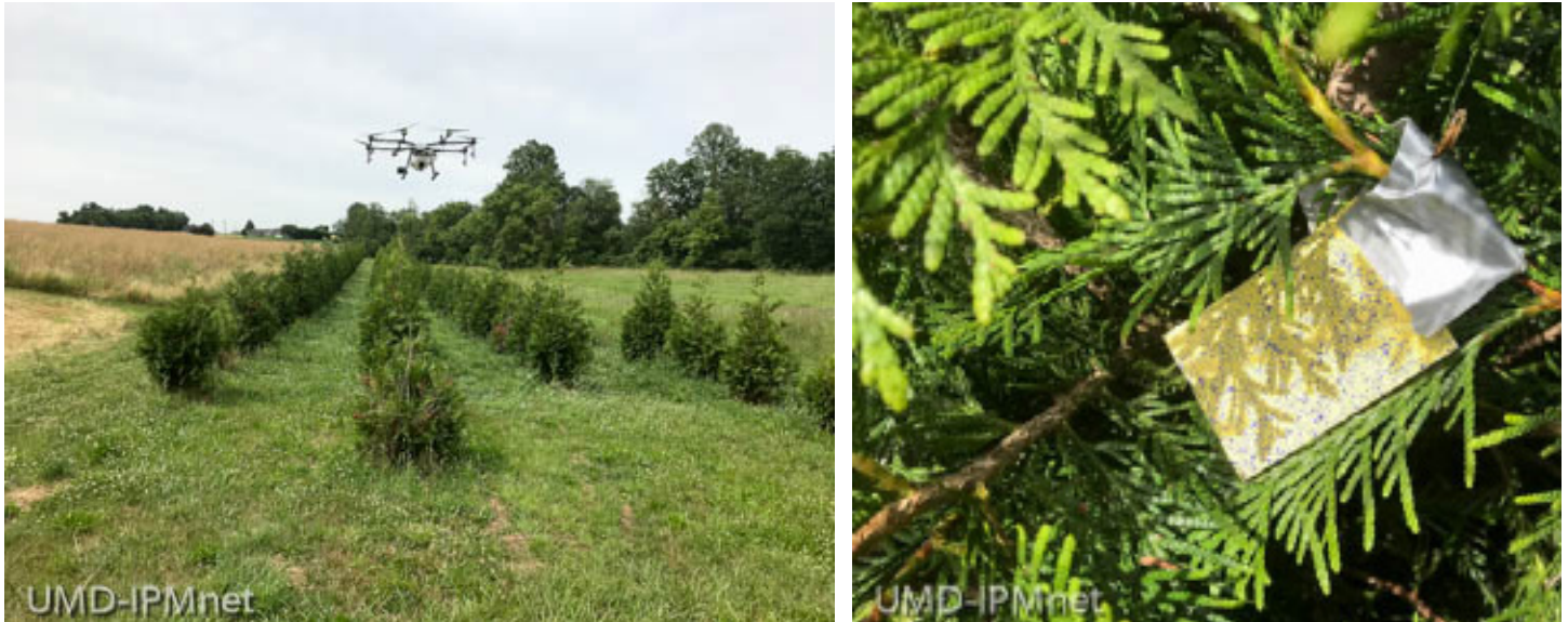
Water is being applied from a drone with a spray tank to test spray coverage on plants using spray indicator cards as shown on the right
