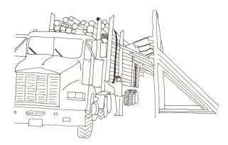
If an unbinding station is not provided, do not loosen binders without support of an unloading machine (clamped over the load) unless the logs are clearly below the bolsters and supported by at least two standards.
