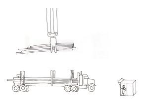
If no driver safety shelter is provided, then the driver should remain in full view of the loader operator while the truck is being unloaded.
