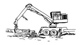
Workers should stay a safe distance away from grappled stems and should never allow grappled stems to pass near them or overhead!!!
