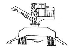
Before climbing to operator's station, check steps, walking, and working surfaces to ensure they are clear of oil, grease, fuel, mud, snow, ice, and debris.
