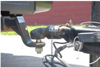
*A bumper pull trailer attached to the hitch.*
