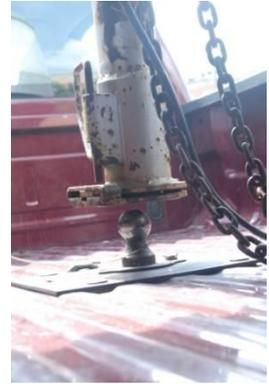
*A gooseneck trailer ready to attach to the hitch.*
