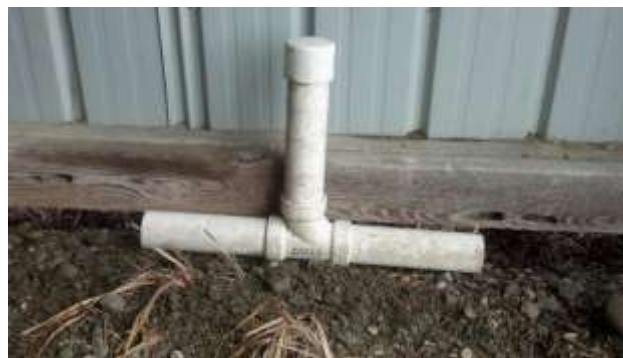
Figure 1. You can make a bait station from PVC pipe
