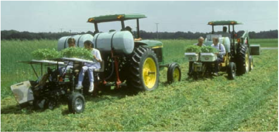
Figure 3. Transplanting tomatoes into hairy vetch mulch using no-till transplanter.
