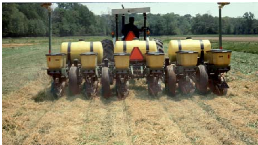
Figure 9. A six-row, no-tillage seeder planting snap beans.
